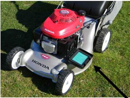
Fit the Air filter from the bottom, clicking into position on top
